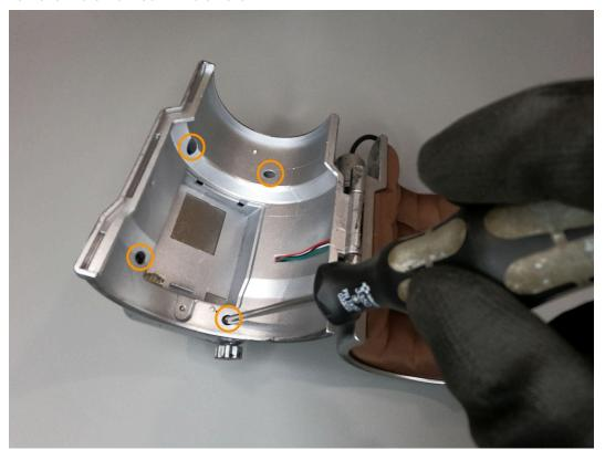
6. Lift the battery compartment away from the front of the Pip-Boy, taking care not to damage any of the wires (which are towards the hinge side)
