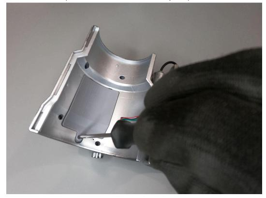
4. Open the battery compartment and lift out the battery, making a note of its orientation and the position of the wires – they're a tight fit when re-fitting the battery
